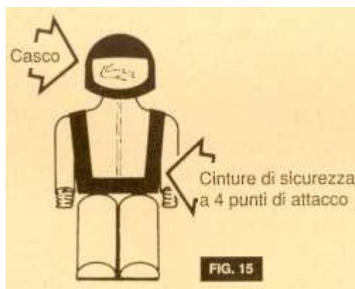
Obviously the anchor points on the aircraft structure must have been chosen to be robust and resistant. Use of this type of harness has particular importance in certain critical flight conditions such as:
